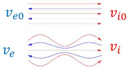
Inherent instability of the current flow: Dissipative response of the electron flow + ballistic (inertial) response of ions
