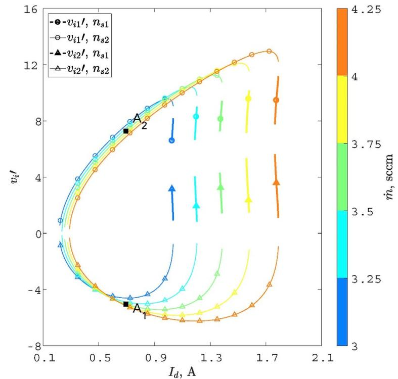
In general: two density roots; each density root generates two values for the velocity derivatives; However some velocity derivatives can be complex; most of the lower density branch does not lead to stationary solution.
