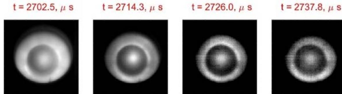
If spoke is an azimuthally propagating mode driven by axial gradients ( $N_i, T_e$ ), axial gradients (profiles) are modified by driven breathing mode!
